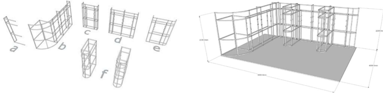
Stand was designed in individual sections so that bays could be used as island displays or as part of the back wall depending on floor space. Sections can be included / omitted depending on the floor space available.
