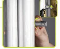
To attach the stand off's, place the rail fixing into the channel on the linear post and twist the bottom section off the stand off until securely in place. Place the graphic into place within the stand off and tighten grub screw until tightly in place.
