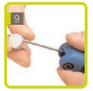
Using a 2.5mm Allen key, unfasten and remove the grub screw from each Poster support.
