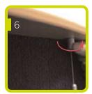
Fasten the adjustment end of each wire kit to the brass inserts on the top.
