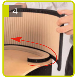
Attach the smaller wrap to the top of the shelf, following the shape of the mount.
